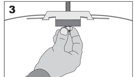
Suspend the assembly from a threaded rod.
